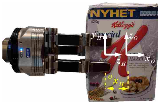
Figure 5: Grasp preshape used for training on the maximum static friction forces and torques, with the corresponding reference frames of the hand and the object used for training.
