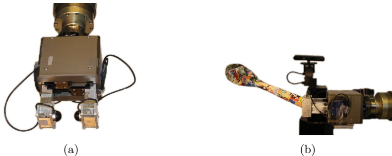
Figure 4: Robot platform with parallel gripper and Optoforce tactile sensors at the fingertips used in our experimental evaluation.
