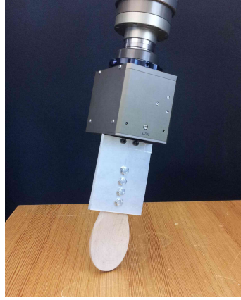
Figure 3: Experimental setup used for evaluating our adaptive control scheme for contact point and surface normal estimation.
