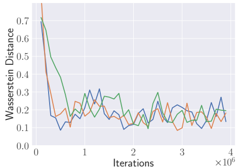
Fig. 4: Wasserstein error of the GAN for several training runs using the same hyperparameters. Note that the model converges rapidly until 500k iterations and stabilizes thereafter.
