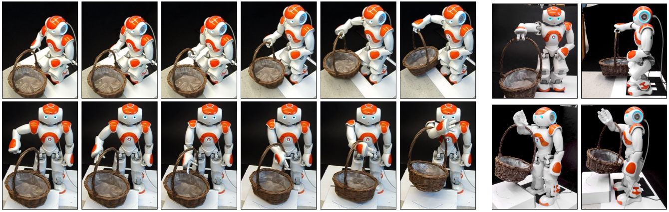
Fig. 6. Examples of the experimental evaluation performed with a Nao humanoid robot. Top row : The robot moves its right hand into approach position and subsequently grasps the handle. It stands up, lifts its arm and lets the basket slide into carrying position. Bottom row : The robot hooks and lifts the basket in one action by performing a grasp frame-parametrized motion template.
