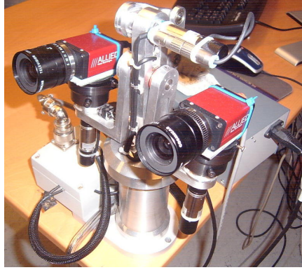
Figure 2.3: Stereo head used in our system
