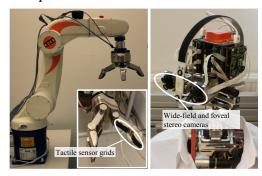
The robot consists of an Armar III, 7 DOF active head and a 7 DOF Schunk Dexterous Hand with Weiss tactile sensors, mounted on a 6 DOF KUKA arm.
