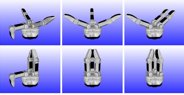
Figure 4: The hand pre-shapes. The top row depicts the  $\mathbf{q}_{\text{open}}$  configurations and the bottom row the  $\mathbf{q}_{\text{closed}}$  configurations. From the left to the right: 2-finger parallel grasp, 3-finger ball grasp and 3-finger cylinder grasp.
