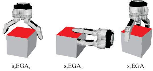
Figure 5: Illustration of the surface-based Elementary Grasping Actions used by the benchmark method [27]. The grasps are targeted at the red surface.  $s_2\text{EGA}_1$  is a two-finger encompassing grasp,  $s_2\text{EGA}_3$  is a two-finger side pinch grasp, and  $s_3\text{EGA}_1$  is a three-finger encompassing grasp.
