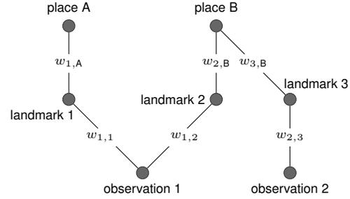
Fig. 1: Example network configuration at one instant, of two observations that are matched to three landmarks, each in turn connected to a place.
