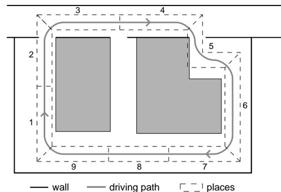
Fig. 2: Environment where the robot drove four laps. The size of the loop is 8 by 10 meters, divided into nine places. The gray area consists of objects the robot cannot drive through.
