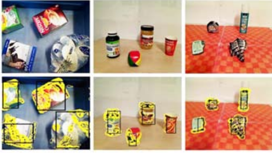
Fig. 2: Results of the visual attention module. The yellow contours indicate the salient regions and the black boxes the regions of interest.
