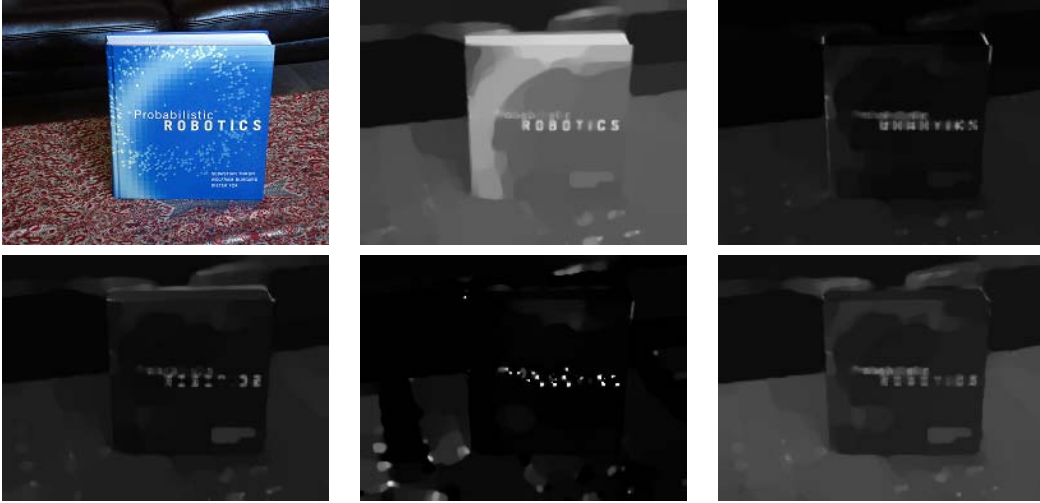
Figure 2.1. A sample image and the corresponding texture feature(threshold on the average total variation per channel per pixel \theta = 2 ). From top left to bottom right: original image, the intensity channel, structure tensor component I_x , structure tensor component I_y , structure tensor component I_x I_y and scaled inverse texture scale.
