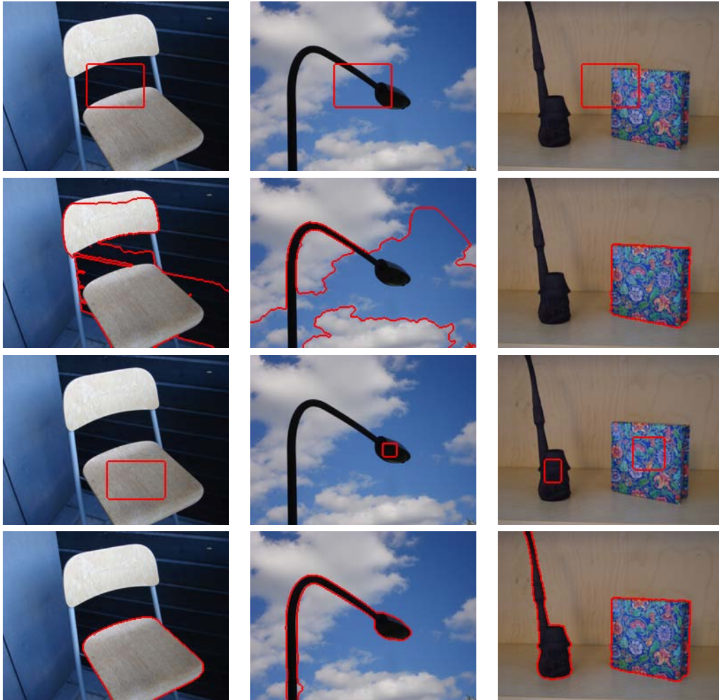
Figure 4.15. The resulting segmentations using \sigma = 16 and different initializations: (top) the default initialization, (second top) the result of the default initialization, (second bottom) manual initialization with the initialization covering a part of the object only and (bottom) the result of the manual initialization.
