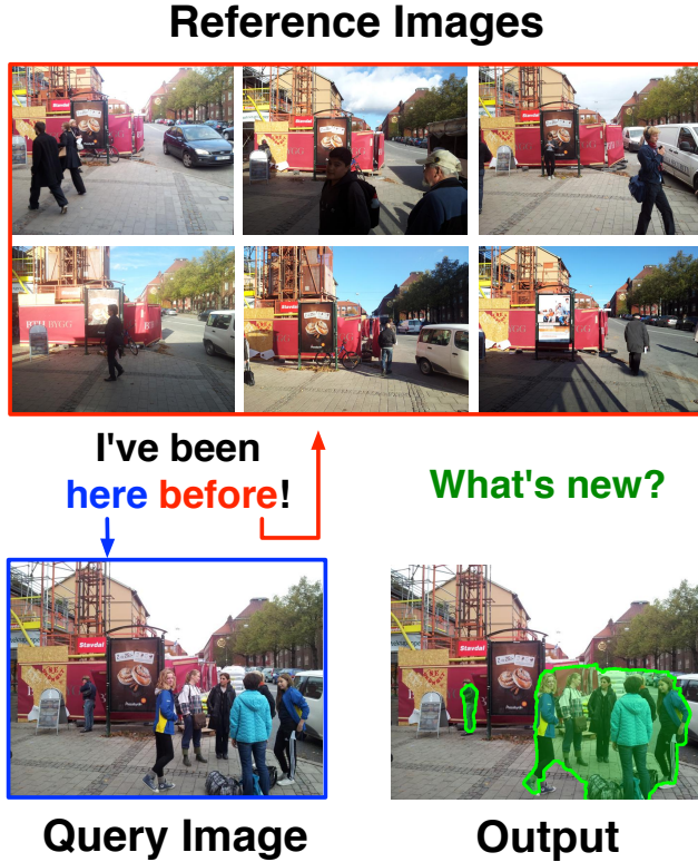
Figure 3: Our system takes as input a query image and multiple reference images. We assume all these images are of the same environment taken from approximately the same view point but at different times. The algorithm segments out objects in the query image which are not part of the environment. The bottom right figure shows the computed segmentation.
