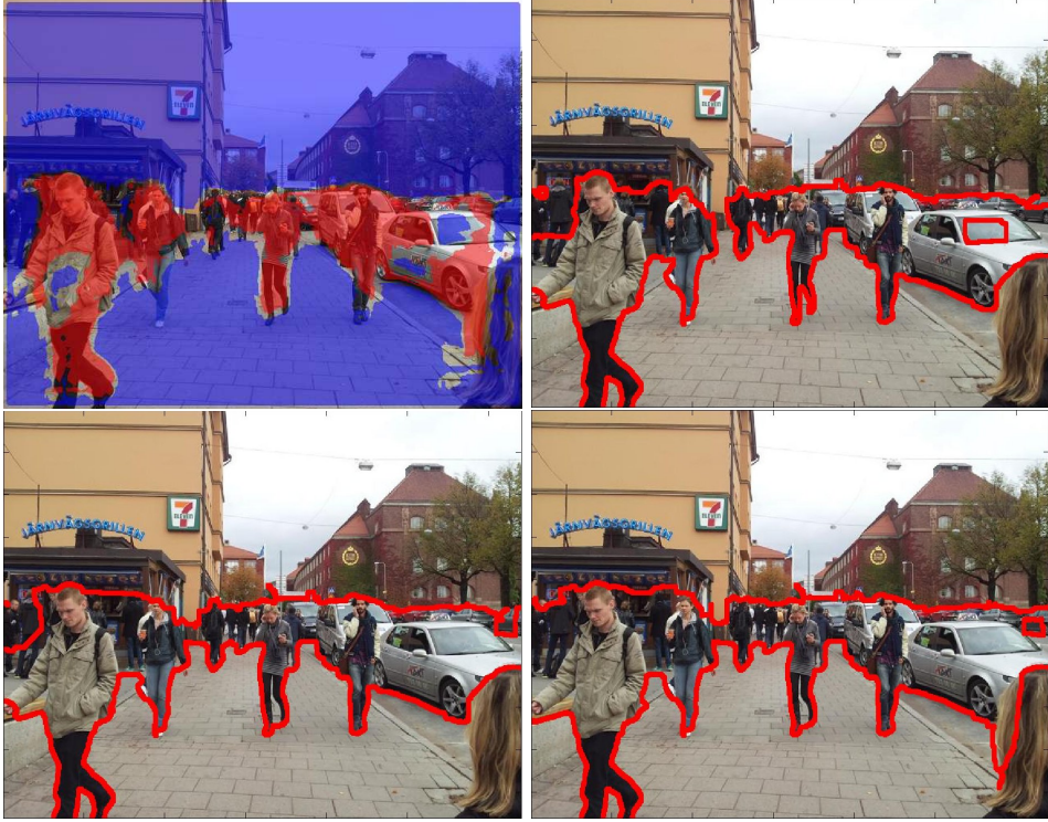
Figure 3: Segmentation results with different class priors: from top left to bottom right: initializing with m_0 = 0.1 and segmentation results using P_H , P_{SF} and P_S class priors. In the figure illustrating the initialization, regions inside blue and red boundaries represent initial estimates of background and novelty regions. The margin m_0 = 0.1 > 0 on \hat{P} (refer to Figure 4) leads to gaps between the regions.
