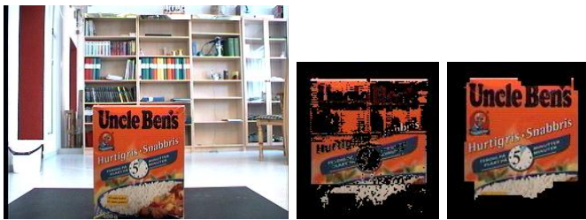
Fig. 3. Left: The original image. Center: The result after image differencing. Right: The result after morphological operations
