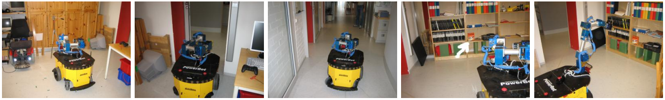
Fig. 8. The robot is instructed to fetch the rice from the living room. It first plans a path and then follows it while avoiding obstacles. Once the goal position is reached, it verifies that the object is still there (marked with the white arrow). The robot signals that it has found the object by pointing to it with the arm.
