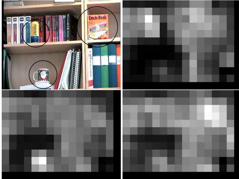
Figure 8: Searching for a soda can, cup and rice package in a bookshelf. Light areas indicate high likelihood of the object being present. Vote matrices: Upper right - soda, lower left - cup, lower right - rice package.
