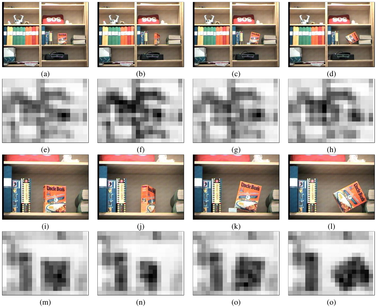
Figure 13: A few example images that demonstrate the outcome of the hypotheses generation process for cases when the rotation of the object relative to the camera changes. It is evident that the rotation around the vertical axis affects the results (figure (b) and (f)) for cases when the object is far away from the camera. A more detailed discussion is provided in the text.
