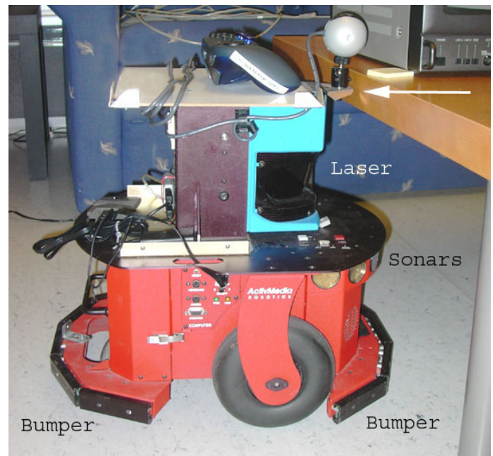
Fig. 1. A Pioneer robot in collision (see arrow in top right corner) with a table. This is not observable by the laser scanner (blue), sonars or the bumper switches since they are vertically displaced compared to the table. At the back of the robot (left in the picture), there is a castor wheel. As the robot drives forward against the table, the weight transfers to the castor wheel and the wheels slip against the floor.
