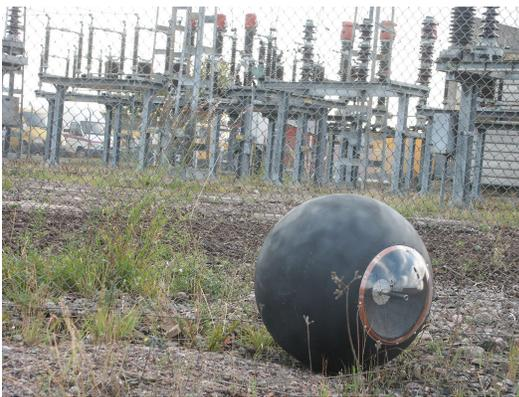
Fig. 1. This Surveillance UGV testbed, developed by Rotundus AB ([www.rotundus.se](http://www.rotundus.se)), will be used in real-world experiments.
