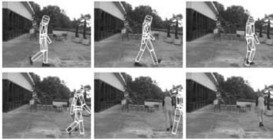
Figure 6.4: How strong is the walking prior? Tracking results for frames 0, 10, 20, 30, 40 and 50, when no image information is taken into account (uniform likelihood function).
