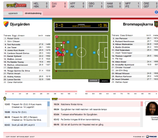
Figure 2: The TRACAB Image Tracking System recovers the positions of moving objects in real-time for instance for publication on the internet (left: “Sportbladet ZOOM” on Aftonbladet’s website) or on television (right: UEFA Champions League).
