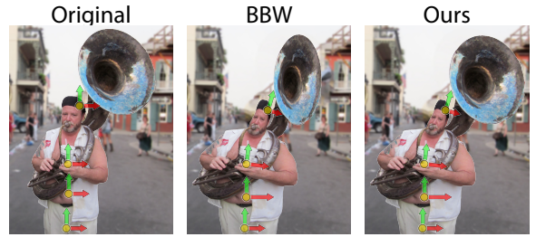
Figure 12: The Sousaphonist in his rest pose (left) is deformed using the bounded biharmonic weights (BBW) of [JBPS11] (middle). Due to local extrema the horn's bell gets an uneven deformation, whereas our local-extrema-free deformation maintains its shape.
