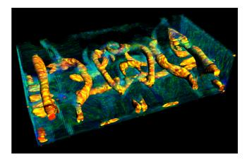
Figure 8: 3D visualization of Benard convection. Benard convection leads to an exchange of heat between a hot bottom surface and a colder top surface.
