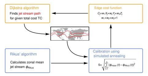
**Figure 2.** Calibration scheme. Before calculating the shortest path with Dijkstra's algorithm, the cost of each edge has to be calculated according to the three terms  $X_j$ ,  $Y_j$  and  $Z_j$ . In order to find the correct weights of the terms, we calibrate them with simulated annealing and using Rikus' algorithm to construct the skill function.
