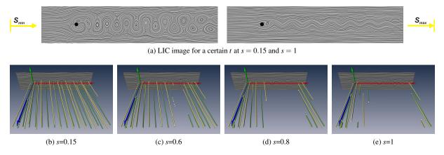
**Figure 7:** Flow behind a circular cylinder: s controls the subtracted constant field, t is the physical time parameter. (a) LIC image for a certain t and two different s, (b)–(e) (x,y,t)-visualization for 4 different s.
