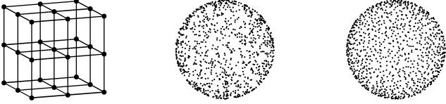
Figure 3. The discrete set of translations \Omega_T is generated as a grid covering a bounding cube. To the left we show an example with |\Omega_T| = 3^3 . The discrete set of rotations \Omega_R is generated by sampling unit quaternions, i.e. points on a hypersphere. In the middle we show |\Omega_R| = 10^3 samples from a uniform distribution and to the right we show the same number of best-candidate samples.
