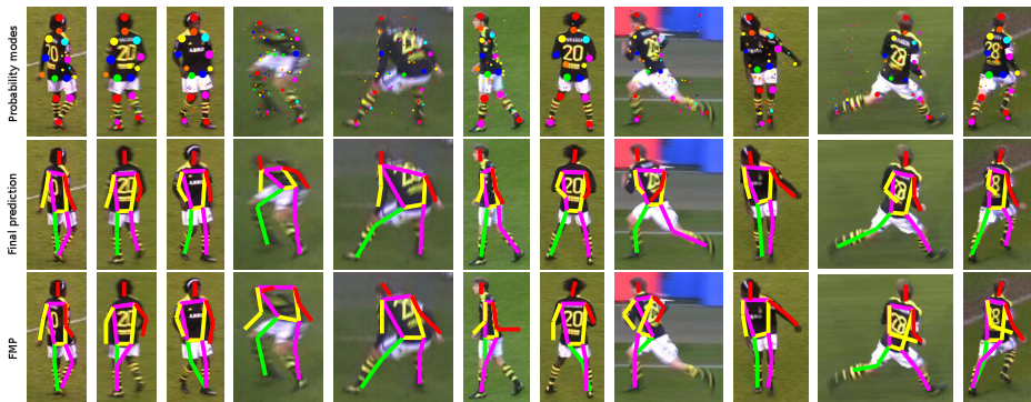
Figure 5: A qualitative comparison of random forests with a state of the art pose estimation method on our dataset. The top row shows the modes of probabilities output from the random forest. A point’s size indicates its certainty level. The second row is the result of inferring the configuration by imposing 2D pose priors. The last row is the result of FMP [24].
