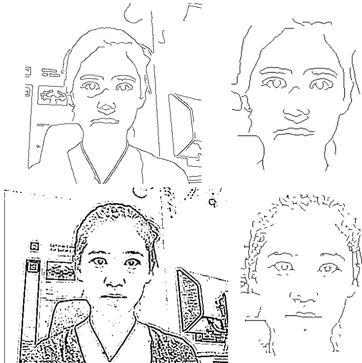
Figure 3.13. Upper left: original Canny edges. Upper right: trimmed Canny edges. Lower left: original Tresset edges. Lower right: trimmed Tresset edges.
