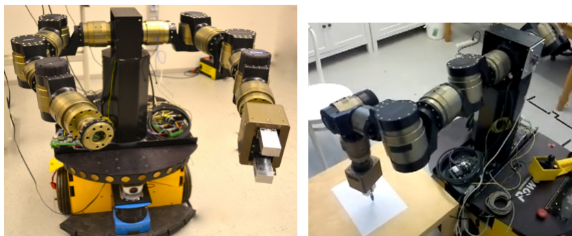
Figure 4.1. Dumbo, the dual arm robot being idle on the left and drawing on the right.
