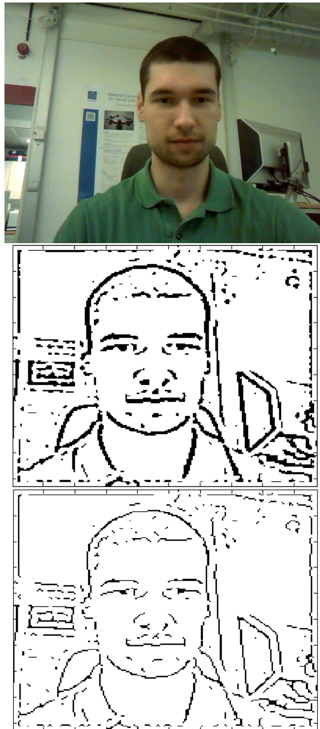
Figure 3.3. Results after applying Gabor filters to only the original scale (before and after thinning).
