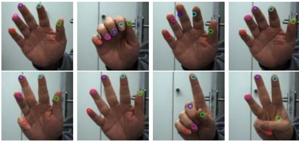
Figure 3. Images of the tracking results. The upper row depicts simultaneous closing of the fingers, while the lower row shows sequential flexing of the fingers. The fingertips are labeled as follows: Thumb (green), index (light blue), middle (dark blue), ring (pink), and pinkie (red).
