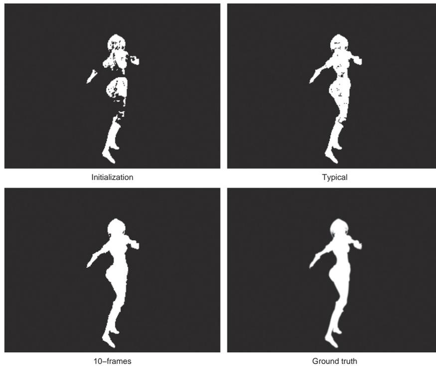
**Fig. 9.** Silhouettes calculated by the foreground detection algorithm for frame #127 of the Kung-Fu sequence (camera #14) for the three parameter vectors. The ground truth silhouette is also provided.
