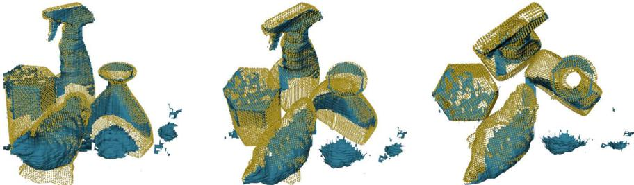
**Fig. 1.** Three views of a typical recognition result obtained with our method. The scene is shown as a blue mesh and the four recognized model instances are rendered as yellow point clouds and superimposed over the scene mesh (see Section 4 for details).
