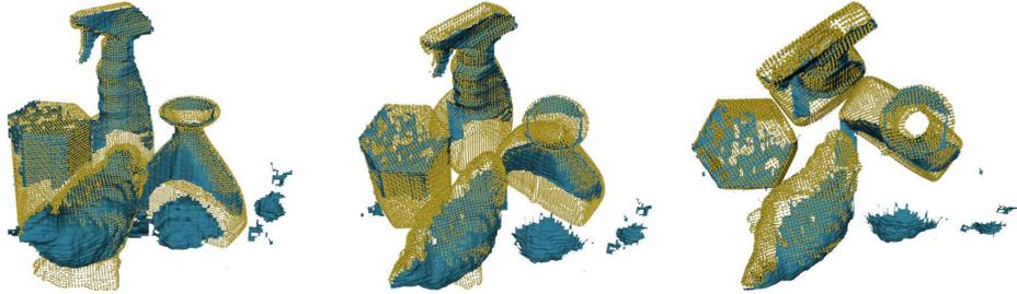
Figure 2.7: Three views of a typical recognition result obtained with our method. The scene is shown as a blue mesh and the four recognized model instances are rendered as yellow point clouds and superimposed over the scene mesh.
