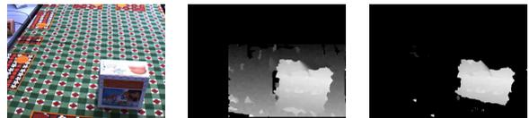
Fig. 7: Results of plane subtraction (Seq. 6). *Left column*: Original color image. *Middle column*: Disparity image of the color image on its left. *Right column*: Remaining object in the disparity image after the plane subtraction.
