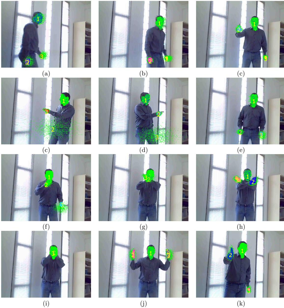
Figure 2.12: Indicative tracking results for twelve segments of the office image sequence used in the previous examples. In all cases the algorithm succeeds in correctly tracking the three hypotheses.
