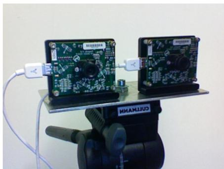
Figure 3.21: The stereo camera system observing grasping activities.
