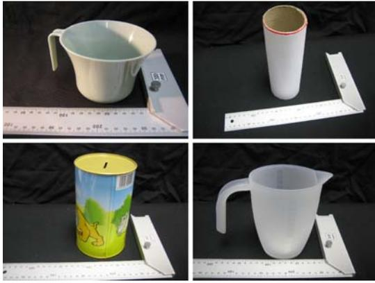
Fig. 6. Cylinder-like objects. Properties (radius x height, weight) from left to right and top to bottom: Cylinder1(110x80, light) Cylinder2(65x215, light) Cylinder3(105x75, heavy) Cylinder4(115x50, light)
