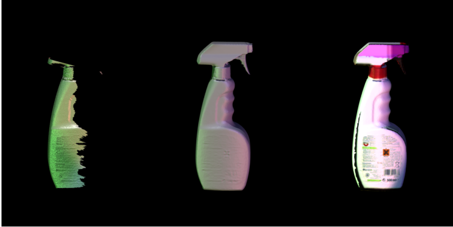
Figure 4.5: Left: Shows the partial mesh as generated from a single scan with the object modeling center. Center: The fusion of all partial scans creates a high resolution mesh. Right: A reduced textured mesh.
