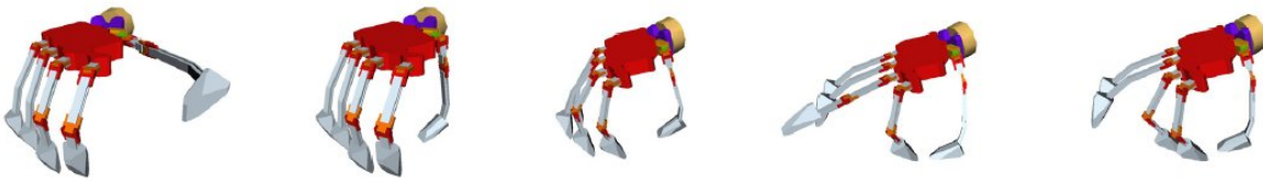
Figure 2.5: Hand preshapes for the five representative grasp types.
