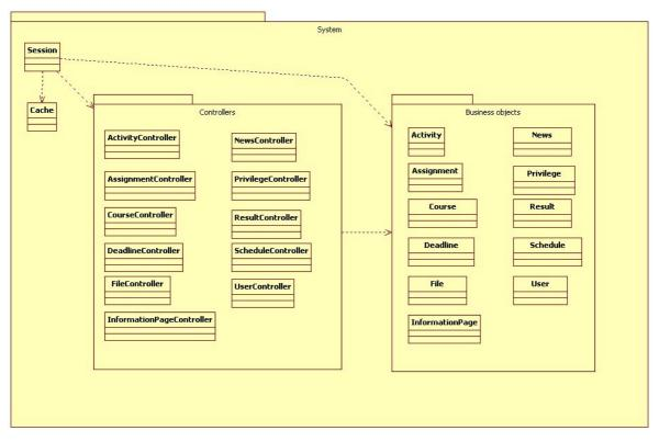
The system can be roughly divided into two packages, one being the controller package. These classes handle loading and saving of information to the database. The other package is the business object package, where the classes represent relevant domain entities such as news, assignments etc. These objects encapsulate all the data of the related entities and are also responsible for all data validation.
