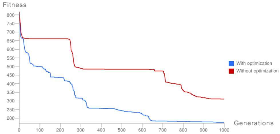
Figure 18: A graph with the average of the top 10 individuals in each generation on the track Comb with and without the genome size optimization (section 4.4.1).
