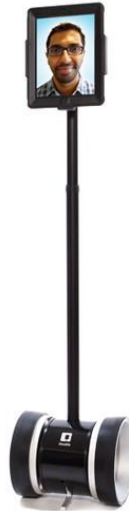
Figure 1.1: An image of the teleoperated robot Double sold by Double Robotics[2]. It is intended to provide distant people with the feeling of presence when engaging in conversations.
