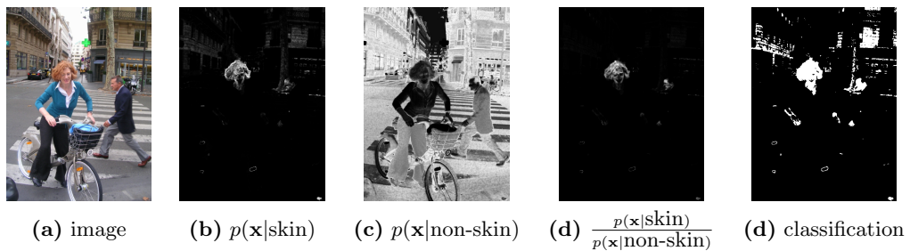
Figure 1: The quantities evaluated to decide via a likelihood ratio test if a pixel corresponds to skin or not. These results were obtained using an rgb representation of color.
