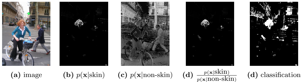
Figure 2: The quantities evaluated to decide via a likelihood ratio test if a pixel corresponds to skin or not. These results were obtained using a hsv representation of color.
