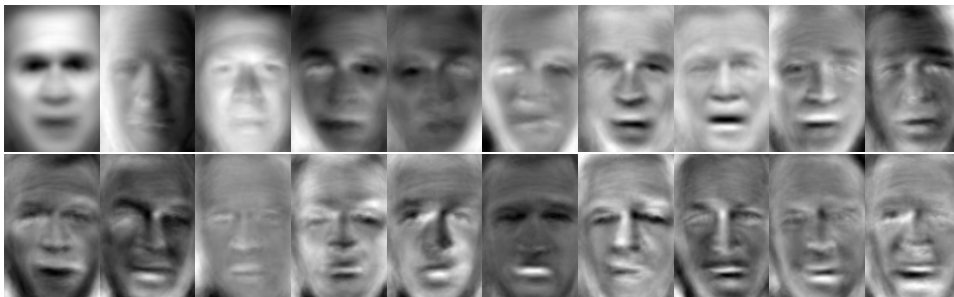
Figure 1: The mean face and the top 19 eigenfaces from the Bush dataset. The top left hand corner is the mean face. While the the rest of the images show the eigenfaces with the largest eigenvalues shown in decreasing order from left to right.
