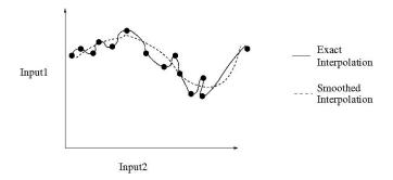
The RBF represented by the solid line hasn N data points and N basis functions (one per dot).
