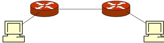
Connect and bring up the network between the host and the router and configure the host with an IP address and static routes according to the topology map.
