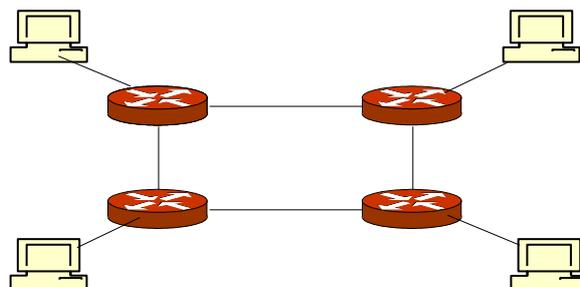
Now connect all four routers in a quad - a square network as shown in the figure. Do not connect the shared network 192.168.15.0/24.
