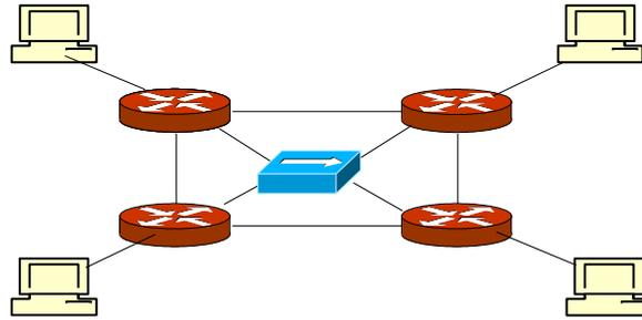
Enable fe-2/0/0 for the shared network 192.168.15.0/24 to study OSPF over a transit network with more than two routers. This network connects all the groups together. Use the addresses assigned in the topology map. Start monitoring with for instance the flags *route* and *packets*.
