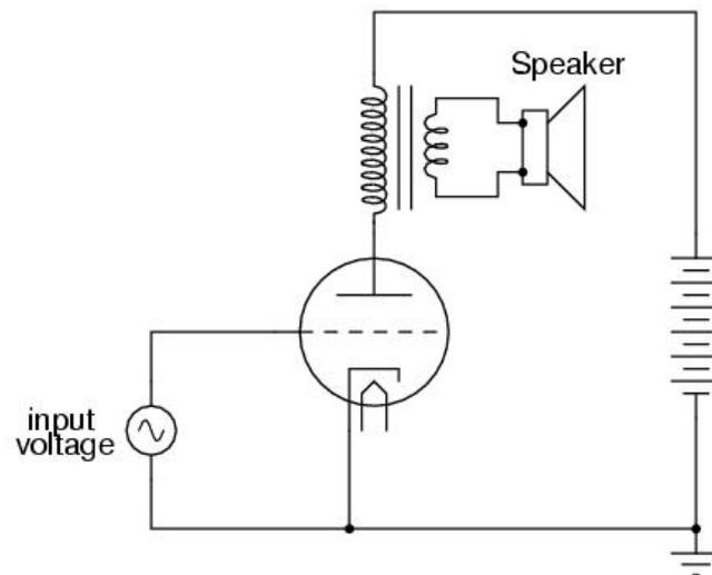
**Figure 2:** Amplifier Circuit
