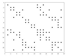
The *pattern* is symmetric: neighborship is a reflexive relation. Also the *values* are the same if the differential equation is self-adjoint. The pattern will change if the nodes are re-numbered. It is important to number such that the elimination process creates not too many new non-zeros.
