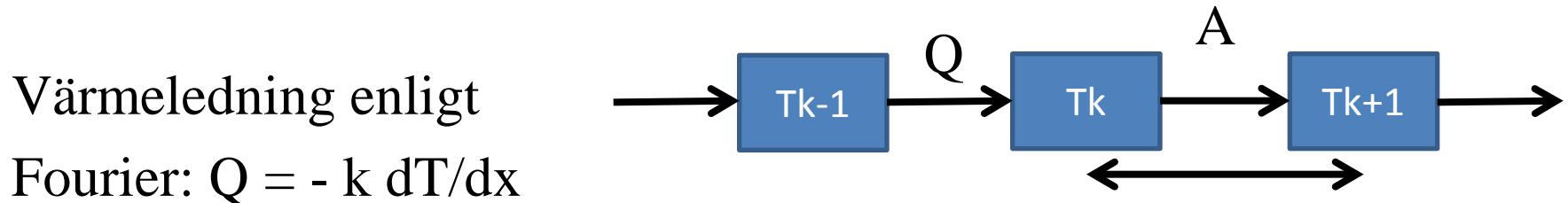
$$\underbrace{\rho A \Delta x C}_{m} \frac{dT_k}{dt} = -\frac{kA}{\Delta x} (T_k - T_{k-1}) + \frac{kA}{\Delta x} (T_{k+1} - T_k)$$
