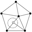
1. loop over all marked cells, for each cell create new nodes at the midpoints of its edges, which gives 4 new red cells, and then
