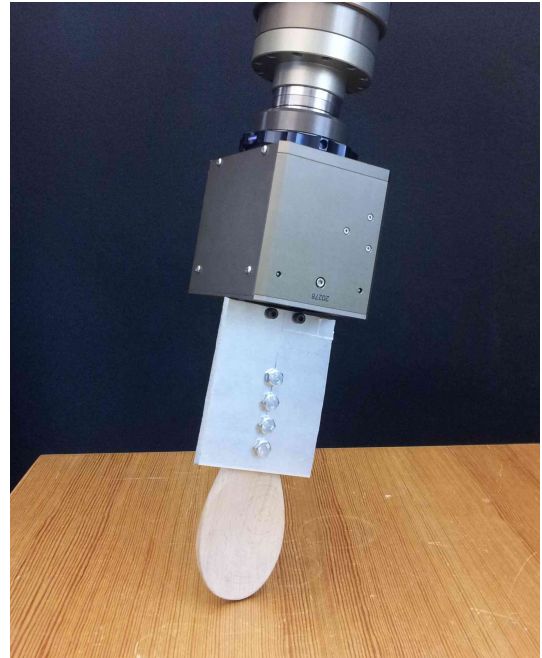
Fig. 3 : Experimental setup used for evaluating our adaptive control scheme for contact point and surface normal estimation.
