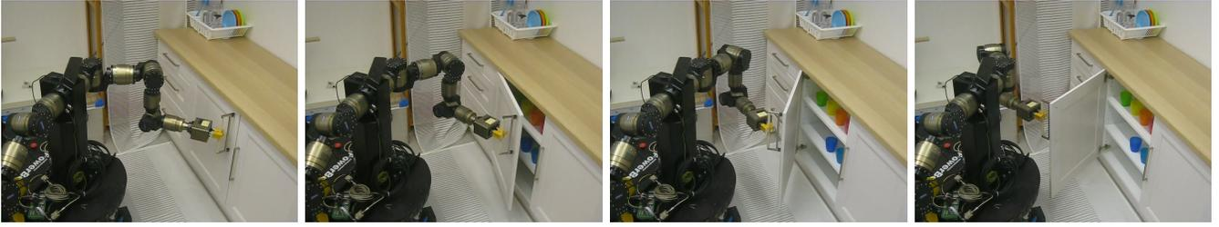
**Fig. 9:** The robot performing the door opening experiment.  $v_d = 0.1$  m/s. The images are taken at  $t = 0$  s,  $t = 1.5$  s,  $t = 3.6$  s, and  $t = 5.7$  s, respectively.
