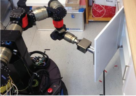
**Fig. 3:** 7 DoF arm of a semi-anthropomorphic robot at CAS/KTH; the figure has been digitally enhanced to mark the joints used for experimental evaluation with red hue
