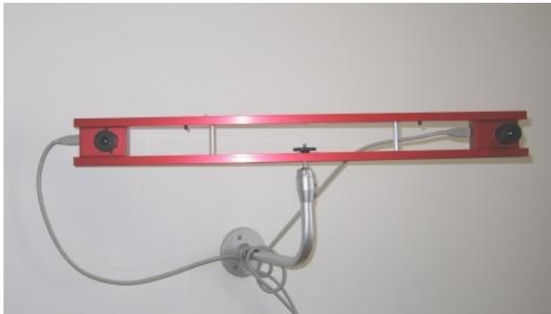
Figure 5.8: 60 cm baseline stereo cameras
