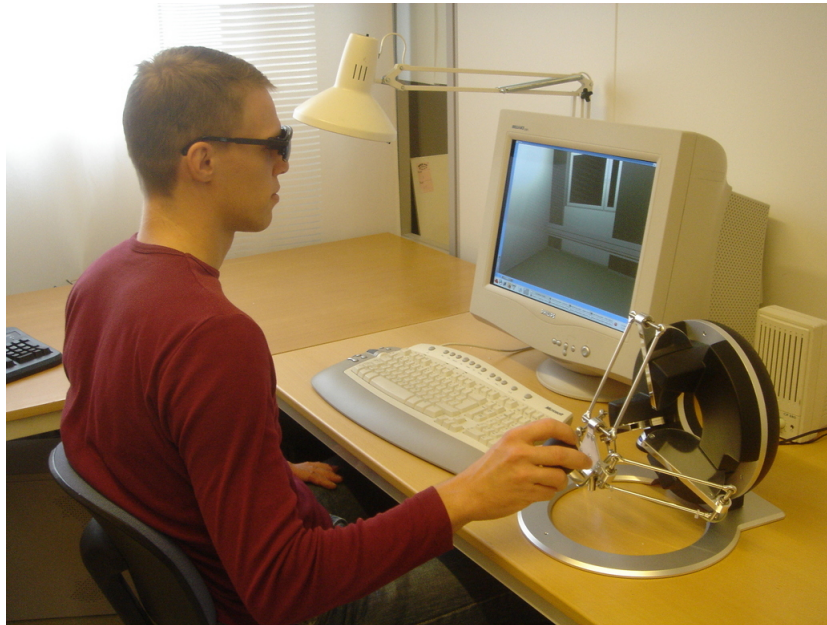
Figure 5.6: Subject using operator station with Omega haptic device and stereo display. Photo by Mattias Bratt.
