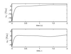
Fig. 6. Input torques responses before reduction
