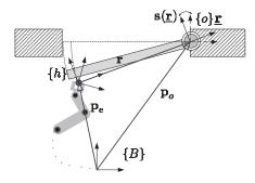
Fig. 1. Kinematics of the door opening
