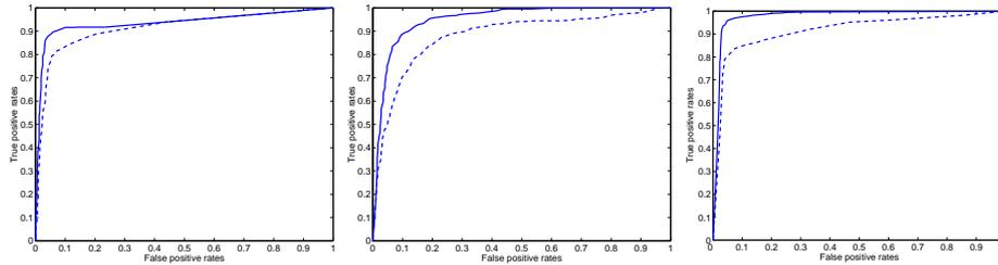
Figure 7: ROC curves for SIFT based (left), colour histogram based (middle) and combined (right) object detection, with (solid) and without (dashed) foveated segmentation.
