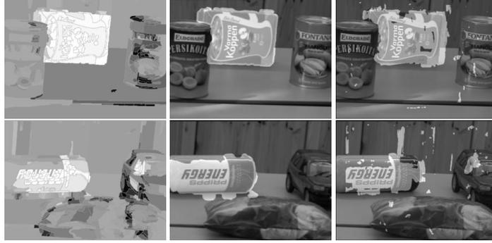
Figure 3: Patches coloured by average foreground priors (left). Foreground segments found using graph-cuts on patches of pixels (middle) and on individual pixels (right).
