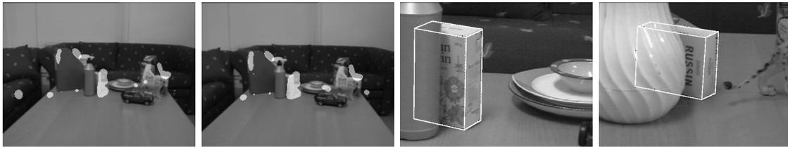
Fig. 7. The effect of occlusions on segmentation and pose estimation.
