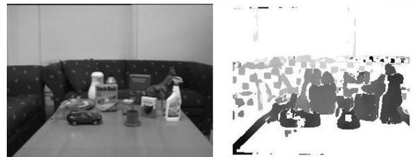
Figure 3: A table-top scene (left) with disparities estimated using sums of absolute differences (right).
