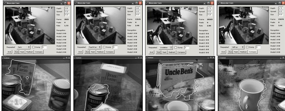
Figure 18: The visual front-end. The top row shows the wide-field view where the visual search selection is made. The bottom row shows the foveal view in which the binocular segmentation and recognition as well as validation is done.
