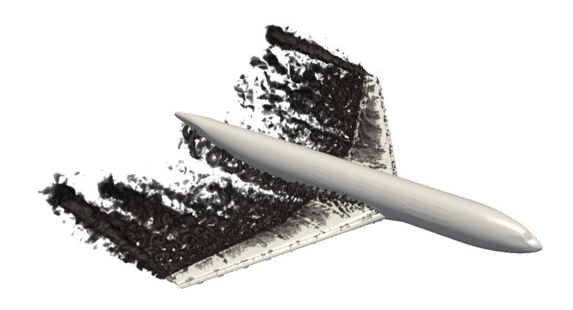
Adaptive mesh refinement with respect to drag/lift for right half plane
