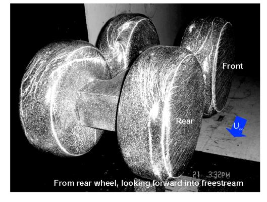
Surface flow separation patterns No boundary layer - inviscid separation
