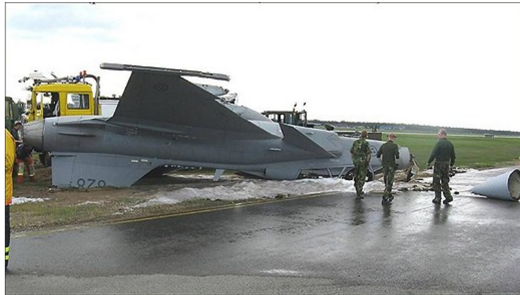
Figure 2.8: The Swedish JAS39 Gripen after crash from longitudinal instability and landing. Note the forward canards supposed to keep the inherently unstable plane in stable flight by rapid active computer control.
