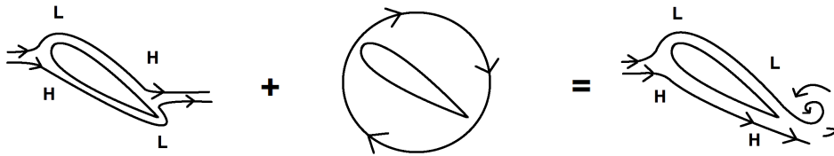
Figure 32.2: Kutta-Zhukovsky theory of lift combining potential flow (left) with large scale circulation, thus changing the zero lift pressure distribution of potential flow to lifting flow by shifting the high (H) and low (L) pressure zones at the trailing edge of the flow by unphysical circulation around the section (middle) resulting in flow with downwash/lift and starting vortex (right).
