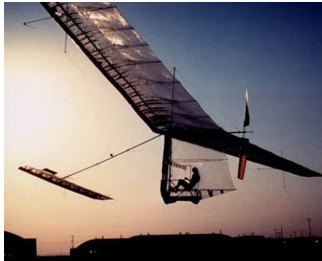
Figure 1.2: The Gossamer Condor constructed by Paul MacCready (wing area of 60 \text{ m}^2 and weight of 32 \text{ kg} ) flew the first figure-eight, a distance of 2.172 meters winning the first Kremer prize of 50,000 pounds offered by the industrialist Henry Kremer in 1959.
