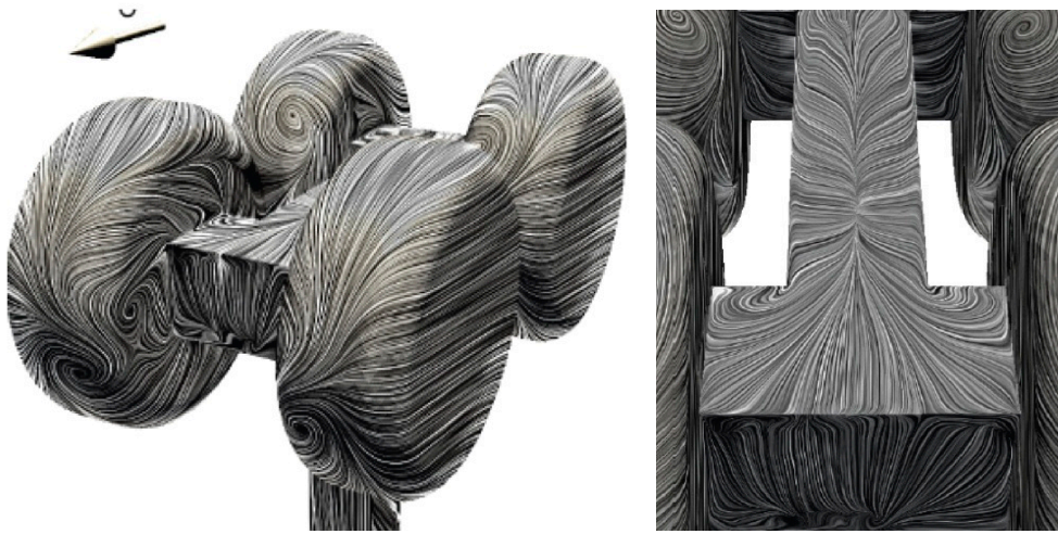
Figure 25.2: Oil film visualization of rotational separation (left) and parallel separation (right).
