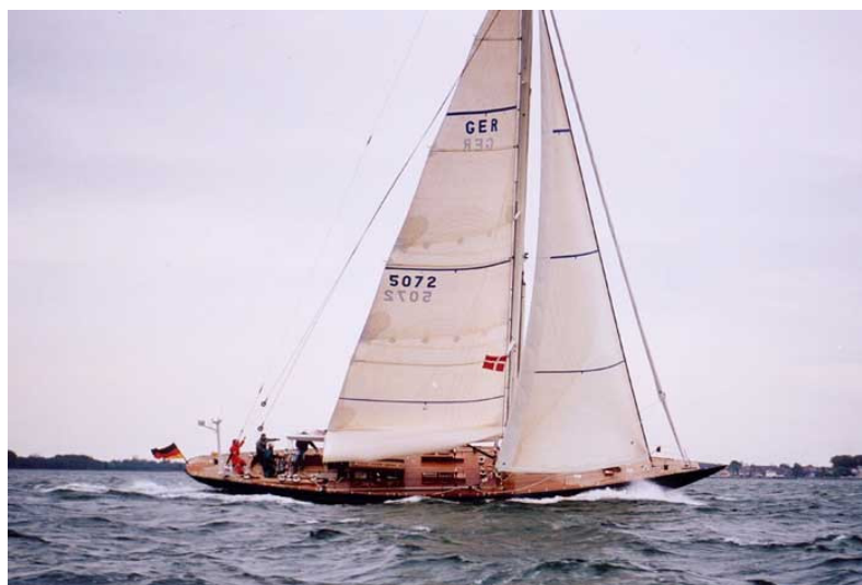
Figure 6.3: Bermuda rig with masthead jib.
