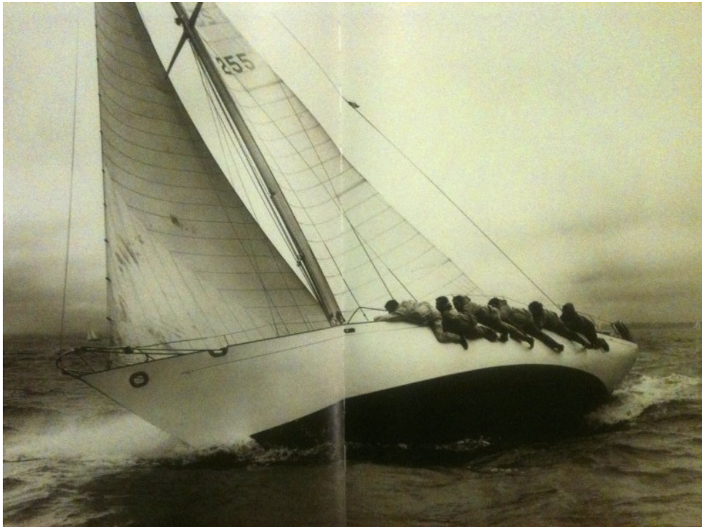
Figure 1: Seeking to balance the heeling on a beat.
