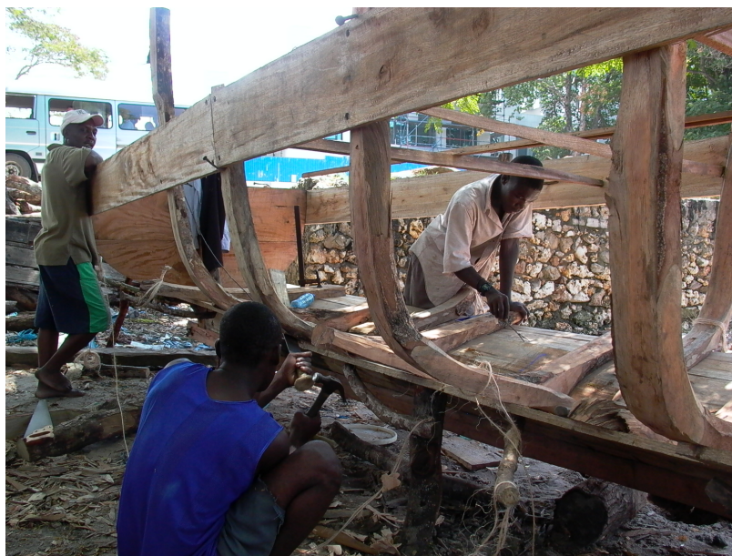
Figure 5.8: Building a dhow on Zanibar in 2005.
